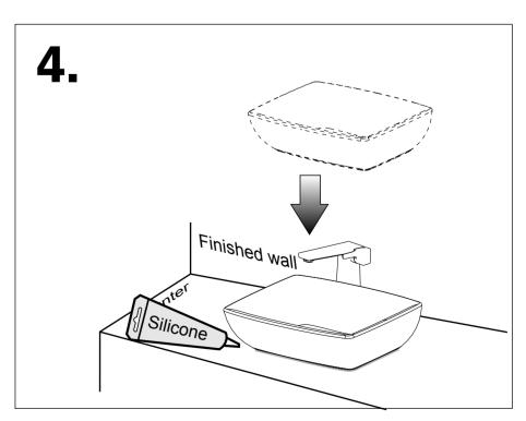
4. Basin taking and follow on position require. To install water supply & waste water outlet set and pop up waste together with basin, proper checking after finish installed, on & off water supply checking, water drainage, water leakage. If no short coming to apply the sealing material with basin's rim. (Sealing material is not provided.)
