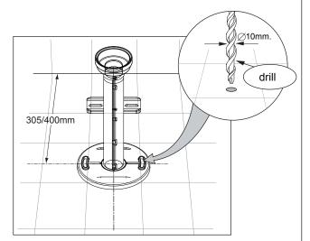
Using Ø10mm masonry drill bit, drill the floor to connect the floor fixing set, follow floor fixing set, follow in the figures.
