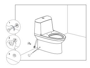
Fix the toilet with the floor by using the screw with the floor fixing set.
