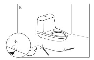
B. Set proprely the VC on the floor, mark the location to be drilled. (the figure just as reference)
