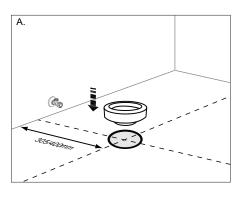
A. Insert the flange into the waste outlet pipe, ensuring that the arrow is pointing toward the floor.
