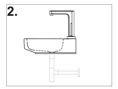
To stall faucet, water supply hose, overflow set completely install with lava.
