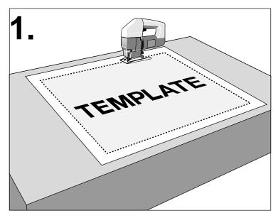
Space preparation for installation as shown. The template placing on the counter with position required following lining by punching
