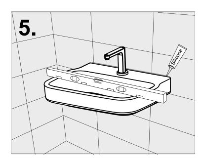
Level check after installation, apply silicone sealant around the lava.(Silicone is not included in the packaging)
