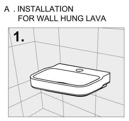
Place the lava to the installing position, mark lava screw locations through the mounting holes.
