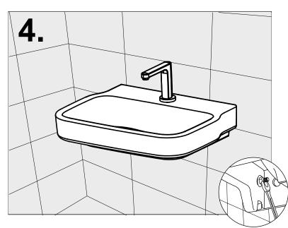
Install the fitted lava to the installed position by using the bolts assembly as picture shown.
