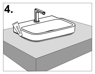
To install water supply&waste water outlet set, proper checking after finish installation, on&off water supply checking, water drianage, water leakage, if no short coming so to apply the silicone sealant around the lava rim. (Silicone is not included in the packaging)
