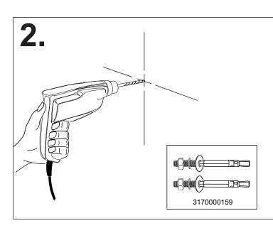
Remove lava from installed position.Drill pilot holes for bolts
