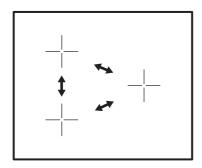
When you set the Power limitation function to **more than 6.0 kW**, power of the hob is divided between two cooking zones in a pair.
